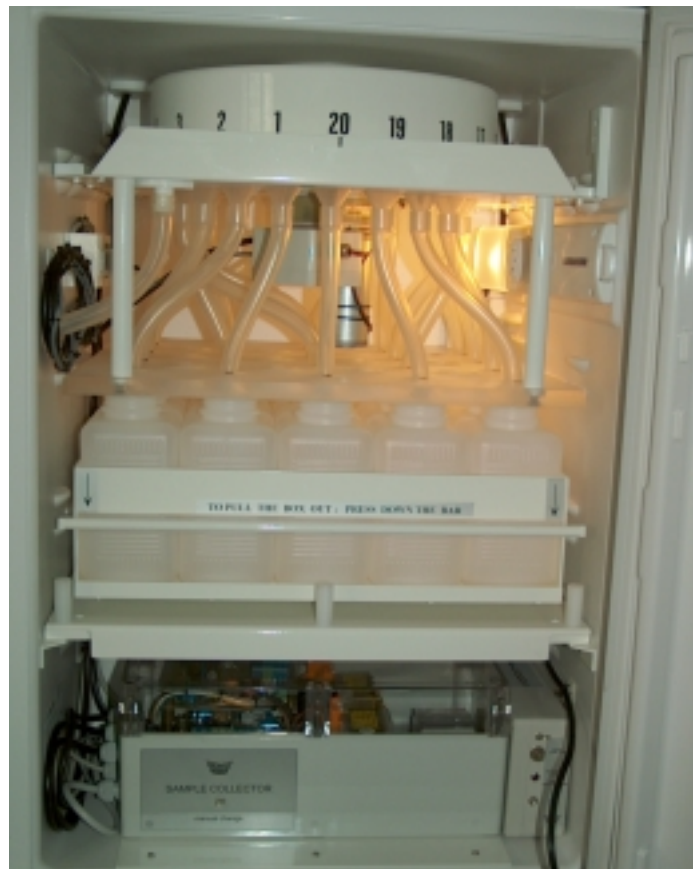
Outdoor – Application: WADOS with a Housing for the Automatic Sample Collector
