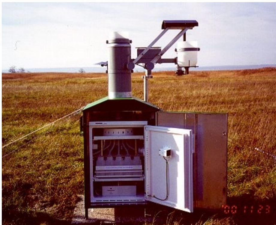
Outdoor – Application: WADOS with a Housing for the Automatic Sample Collector
