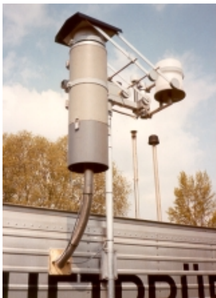
WADOS mounted on the roof of a Container
