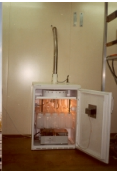
Automatic Sample Collector inside of a Container
