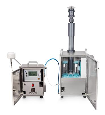
During operation, after the completion of one sampling period, a forcibly guided handling system takes a cassette with a clean filter from the storage magazine and inserts it into the sampling position. Simultaneously, the filter cassette with the dust-laden filter is removed from the sampling position and inserted into the magazine for exposed filters. The use of a Geneva drive prevents any obstructions of the complex movements of the components.
