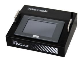
The Fidas® system is offered in different versions in order to be able to use, depending upon application, a low cost solution for the reliable indoor/outdoor quality measurement (IDQ/ODQ). Each Fidas® system is equipped with one LED light source with high light stability and long lifetime.
