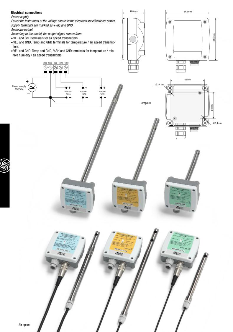
HD29V3T...: Active transmitter for measuring air speed in ducts, 0...10Vdc output. AlSI 304 steel probe, diameter 12mm, compact unit HD29V3T0... version with probe joined to the electronics enclosure, HD29V3TC... version with probe connected to the electronics through a cable. Air speed range 0.05...1m/s 0.1...2m/s - 0.20...10m/s - 0.20...20m/s selected by jumper. Power supply 16...40Vdc or 12...24Vac. Air probe operating temperature -10+80°C.
