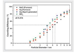
Efficiency of the CPC 5.414, measured with four different particle materials. A Faraday Cup Electrometer was used as reference (Rennecke 2010).
