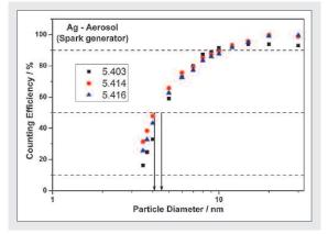
Counting efficiency as a function of particle size, measured with silver particles, for the CPCs 5.414 and 5.416. Both models feature the same new detection head. The efficiency of the mobile CPC 5.403 is shown for comparison. Data from Rennecke 2010.
