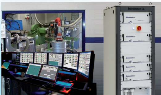
Example: engine testbench with EGAS turnkey system
