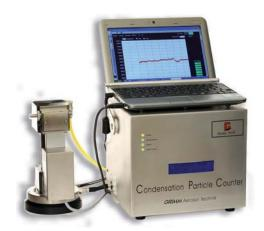
GRIMM DMAs feature the Vienna-type design (Reischl et al. 1997, Winkelmayr et al. 1990), well known for highest resolution and lowest diffusional losses even for small particles. GRIMM offers a flexible design of the Vienna-type DMA with two electrodes of different length to accommodate a variety of experimental needs.
